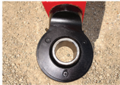
NA COUPLING EYE FOR EITHER 1.5" OR 2" DRAW PIN (Interchangeable)
