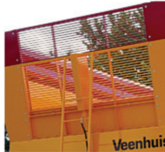
HYDRAULIC SLIDING FRONT GRILL PLATE (Bottom-up sliding shown. Also available Top-down)
